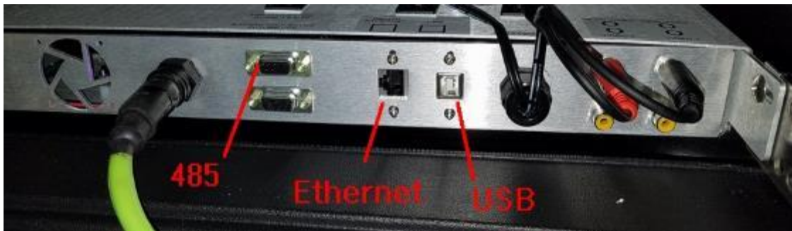
Figure 15: CON-1050 with internal VDSL modem
