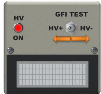
Indicator will blink then remain illuminated indicating thrusters are powered. If Indicator blinks and goes out this indicates an issue. Refer to manual and troubleshooting guide for details.
