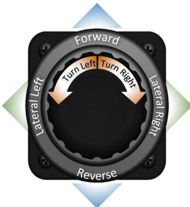
Move Control joystick in each direction and verify associated thruster activates.
