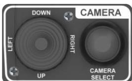
Press Camera Select to cycle through available cameras. Verify video is displayed on monitor.
