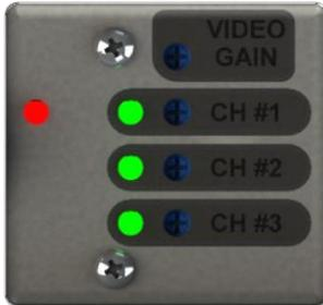
The image to the left shows the Video Amplifier adjustment section. The red Low Voltage (LV) light indicates low voltage is good and the green lights indicate video signal.
