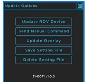
Send Manual Command: This option is used to change factory settings not available through the overlay. This option is only to be used with direct assistance from Outland Technology.
